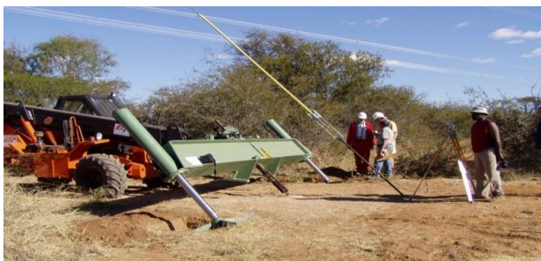
Figure 11-3: Mobile Proof Load Test Rig
