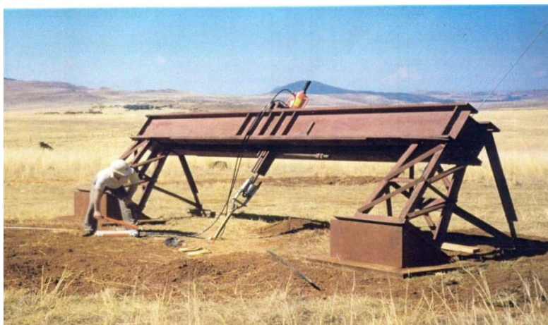
Figure 11-2: Conventional Proof Load Test Rig
